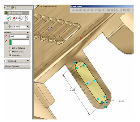
24. Now we can refold the tab - % Hand out created part Sheet Metal 🗞 🖆 🎼 by using the Fold tool on the WERCZH/CA DD 11100 30 IJ Fold3 Sheetmetal tool bar, **VX**? returning the tab back to its original shape. Fixed face: Face<1> Bends to fold: Ø, JogBend1 JogBend2 Collect All Bends adde
