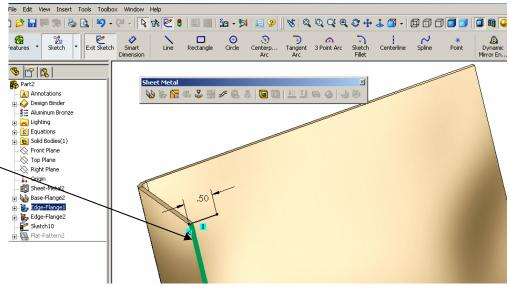
8. Select the Miter Flange button and the size of the flange is selected from the sketched .500 inch line. The first edge is also selected from the edge that the line was sketched from.
