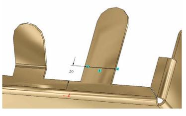
15. Select the Jogged tool. The first requirement is to select the fixed face. Then you can set the jog offset, the dimension position the jog position and the angle of the jog.
