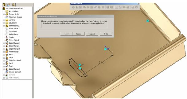
Apply the Geometric Constraints and Dimensions for your requirement. And finish
