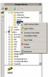
19. Drag and Drop the louver to the surface that you would want the forming punch to come from. (The first surface that the forming punch would contact)
