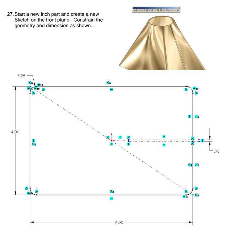
The rectangular geometry on the right side of the sketch is used to create and center a gap in the sketch geometry. Finish sketch and Exit Sketch.
