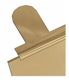
12. Next we need to create a sketch on this tab that will start and stop on the far edges of the tab. The sketched line can either be perpendicular to the edges or at a selected angle. I placed my line .375 inches from the miter flange. Exit sketch and select the Sketched bend tool. The first requirement is selected the Fixed Faces, then you can set the bend angle requirements.
