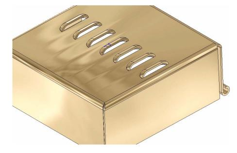
21. Now we will use the Unfold tool to unfold the jogged tab. Select the fixed face and then select the two folds that need to be unfolded.
