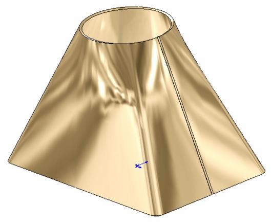
31. Select Flatten on the Sheet Metal toolbar and the sheetmetal transition that we just created will turn into a flat pattern layout.
