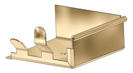
16. Add a 2.50 inch Edge Flange on the side of the base part that we haven't used yet.
